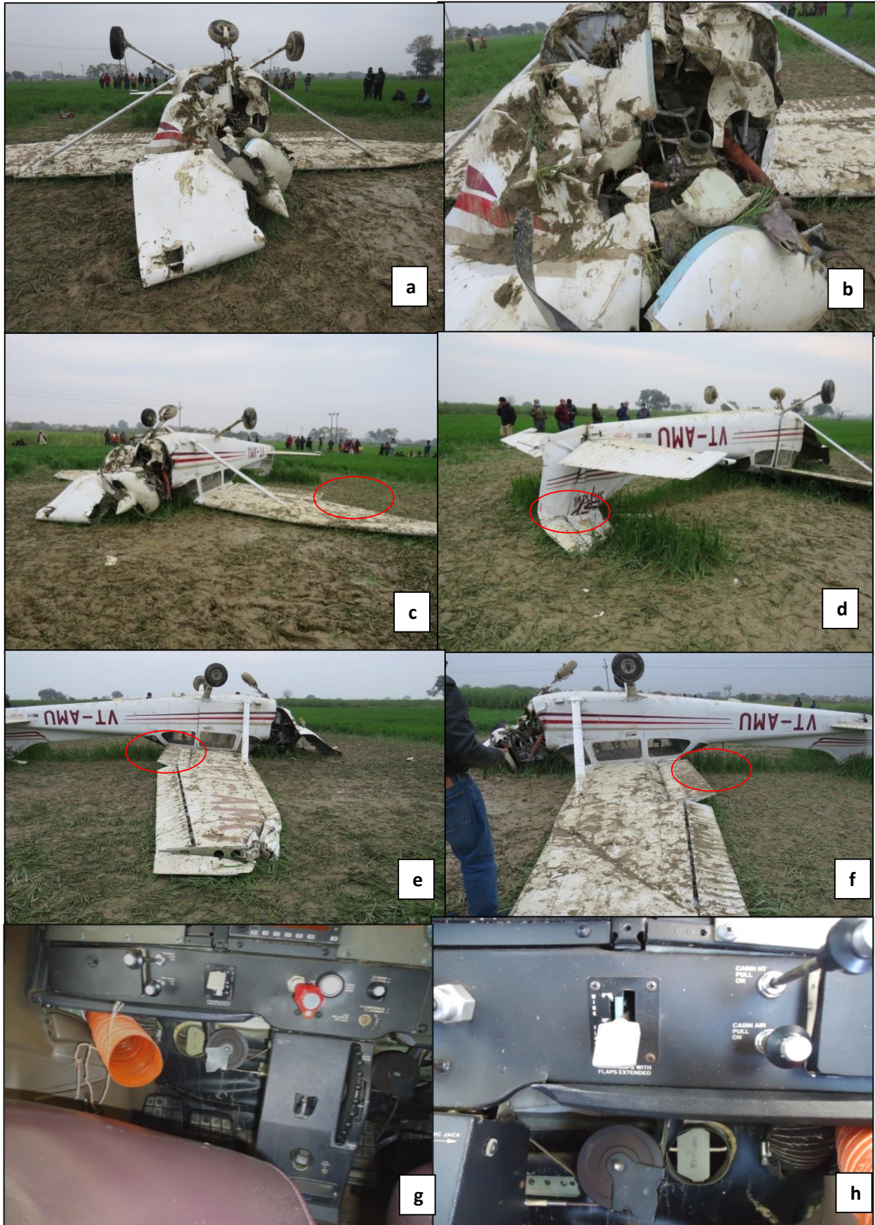
Figure 2 (left to right): a-Damaged Aircraft upside Down; b-Damaged Nose Portion; c-Bent Starboard wing; d-Bent Ventral Fin due to weight; e-Aircraft Left Flap extended position; f-Aircraft Right Flap extended position g-Flap Selector Switch in 100 Position; h-Throttle in Full Power Position
